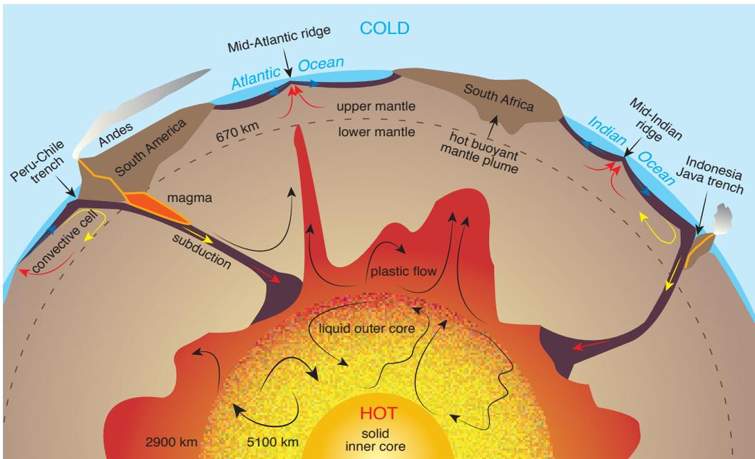
Internal cutaway showing convection in the liquid outer core that generates our magnetic field and convective plastic flow of hot, solid mantle rock that drives plate tectonics
